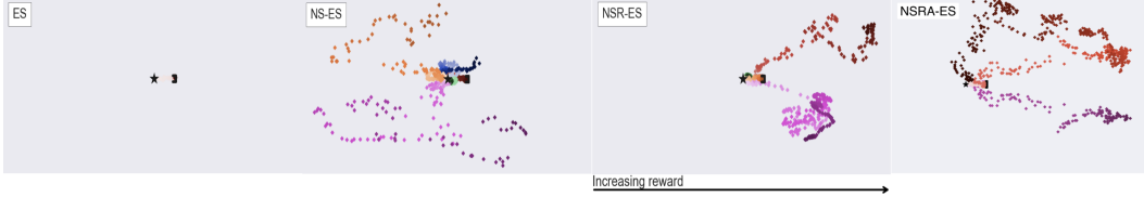
Figure 2: ES gets stuck in the deceptive local optimum while NS-ES, NSR-ES & NSRA-ES explore to find better solutions. An overhead view of a representative run is shown for each algorithm on the Humanoid Locomotion with Deceptive Trap problem. The black star represents the humanoid’s starting point. Each diamond represents the final location of a generation’s policy, i.e. \pi(\theta_t) , with darker shading for later generations. For NS-ES, NSR-ES, & NSRA-ES plots, each of the M = 5 agents in the meta-population and its descendants are represented by different colors. Similar plots for all 10 runs of each algorithm are provided in SI 6.9.
